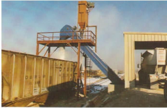
Soda Ash-Unloading 80,000 lb. (trailer & pup) in 20 min. (120 TPH)
