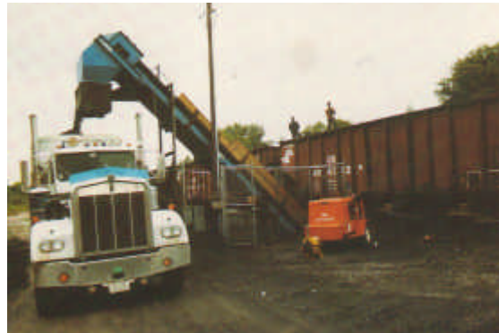
Boiler Coal-Loading a 24 Ton Trailer in 4 minutes (360 TPH).
